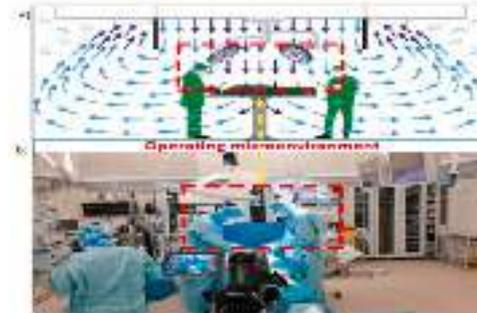
Fig. 2. (A) Schematic outline of airflow from a LAF unit, and (B) example of a vertical laminar LAF hood. (C) Hospital in production (medical laboratory) during the operating environment (0.25).
